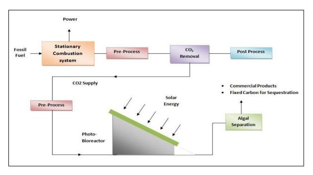
Fig.2- A simple concept for a microalgal-based carbon capture scheme
