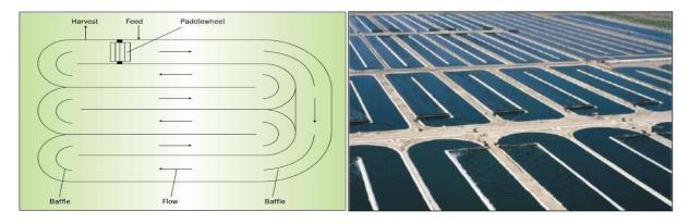
Fig.3- A raceway pond system
