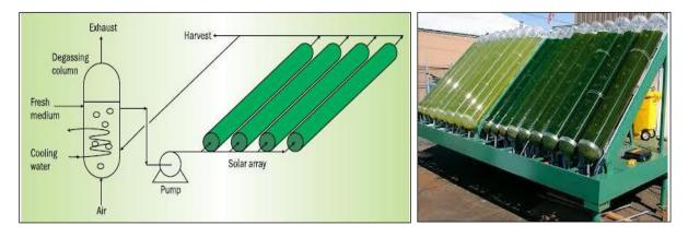
Fig. 4- A closed photobioreactor (PBR)
